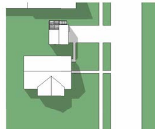
D Garage Prototype For parcels with limited rear yard space, places the ADU above an existing garage.
